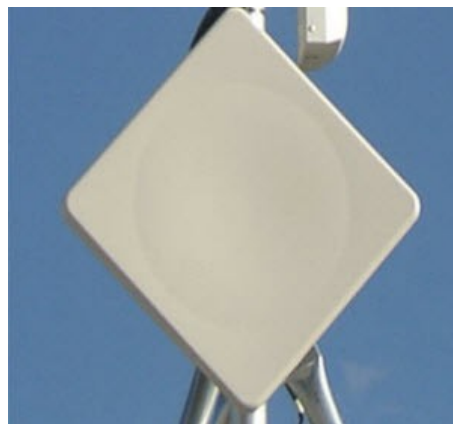
Figure 4 Panel antenna uses for Point-to-Point applications.
